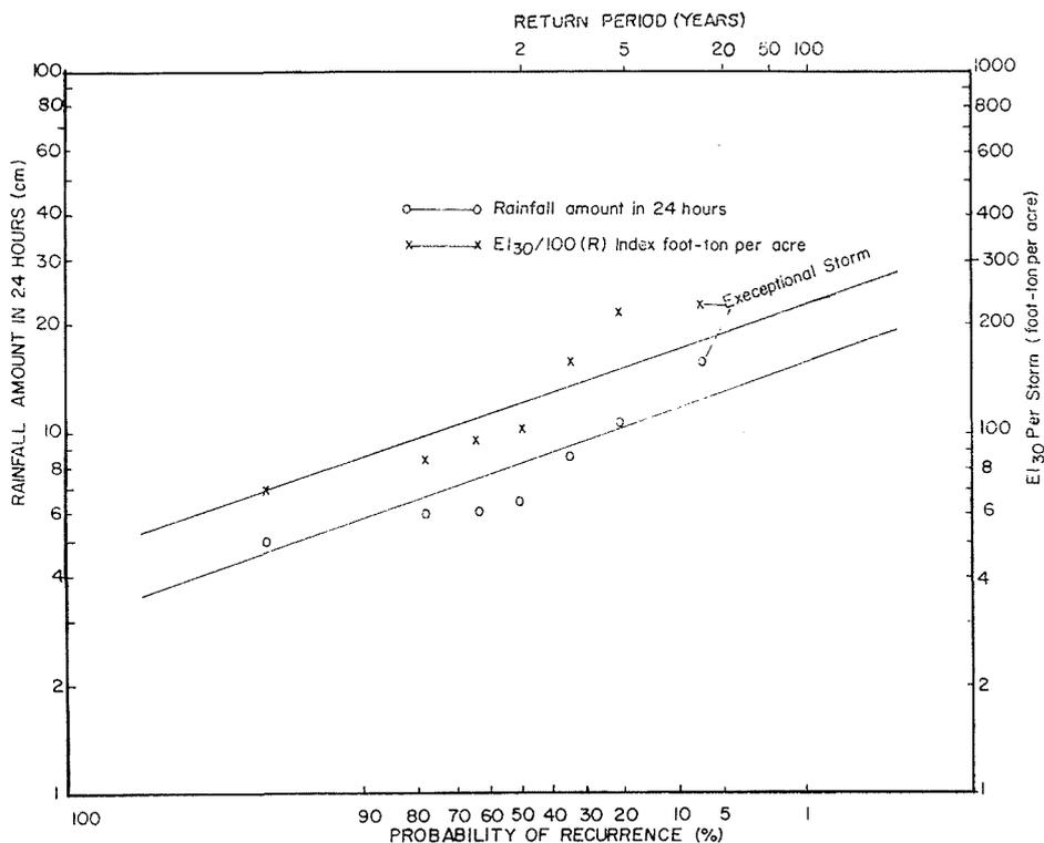
FIG.2 Return period and frequency of the EI<sub>30</sub> index (R) and of rainfall intensity for a storm at Ibadan (modified from Lal et al., 1980).
