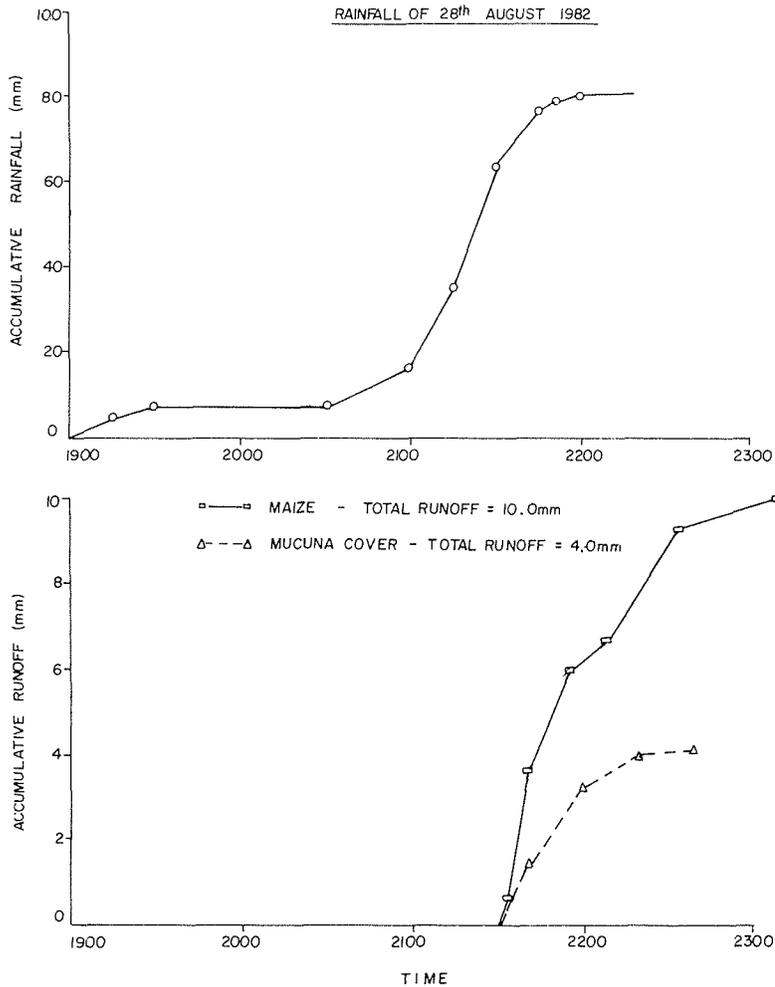
FIG.3 Runoff hydrographs from two catchments on alfisols growing maize and *Mucuna* cover.
